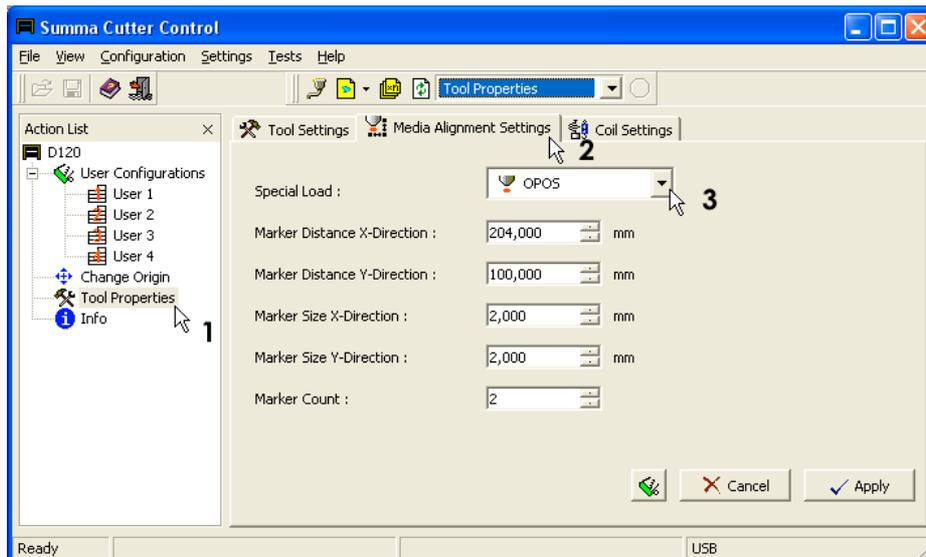
3. Enter the value for the **X-Distance**. X-Distance is the distance between the two markers along the X-Axis (1).
