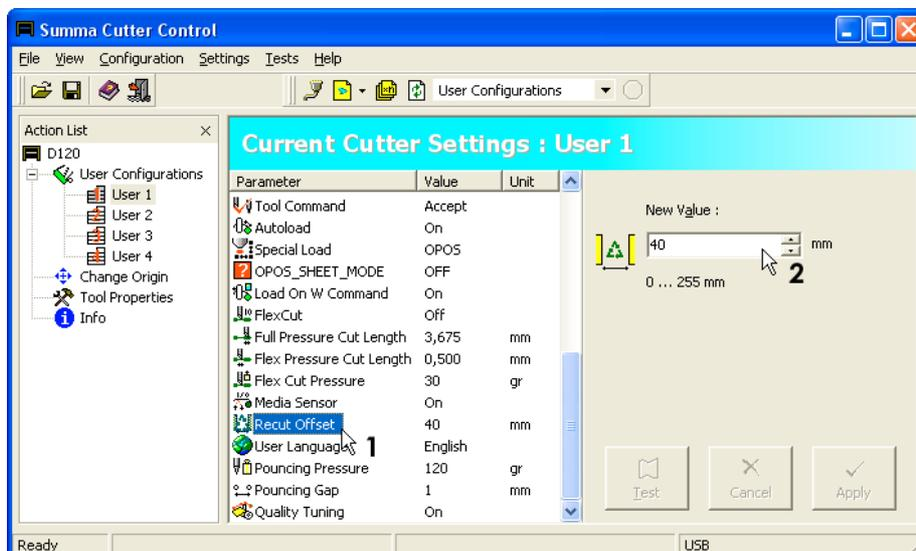
4. Set the **RECUT\_OFFSET** parameter in the **New Value** window to equal the distance between the last marker on the first graphic and the first marker on the next graphic. This setting reflects the distance between two graphics.
