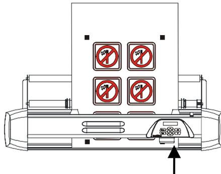
**The sensor must be directly over the Origin marker.**
